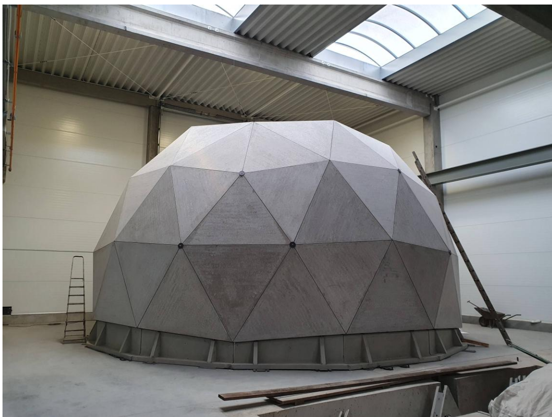
Figure 9. Assembled dome at testing site prepared for initial loading for stiffness analysis.
